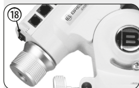
Fig. 20: Switching on the mount electronics
